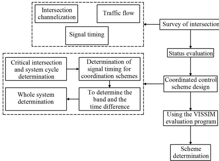
Fig. 2. Signal coordination control system design flow
