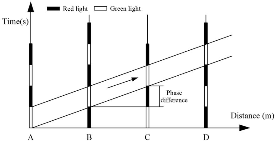
Fig. 3. Time distance graph of four adjacent intersections
